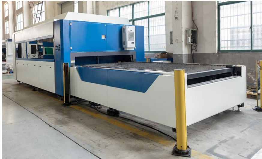
AWE 6kW CNC Fibre Laser (1500 x 3000)
